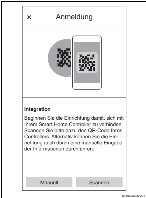
Bild 11 QR-Code am Bosch Smart Home Controller scannen (Bosch Smart HomeApp)
